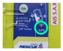
This green LED is flashing after a successful position fix of the internal GPS receiver. The flashing lasts as long as the device is set to Distress Alert mode and as long as GPS signals can be received with sufficient signal strength. Conducting a device test by pressing the TEST button will also result in a flashing of this LED, as soon as GPS has position fix. Good GPS reception will be achieved with a free view to the sky, please have this in mind
