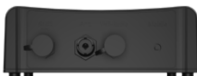
Sideview with: ext. GPS | VHF Ant. | VHF Radio
